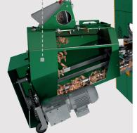
The KWB Multifire can optionally be equipped with a 175 I large hopper that is automatically filled with wood chips from the storage room. This means that the conveyor system has to start less frequently thus minimising the amount of noise and power consumption. If required, the hopper can be filled manually. Including hopper: 10 years full warranty\* on the conveyor system!
